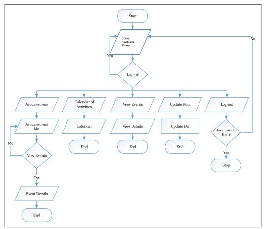
Figure 5. Flowchart for Ubiquitous Notification Application for user
