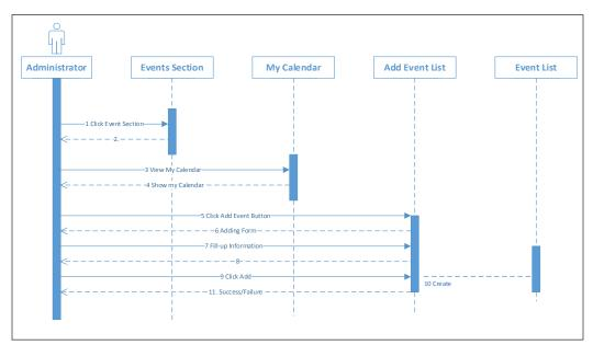
Figure 14. Sequence Diagram for Administrator's Event Section Setting
