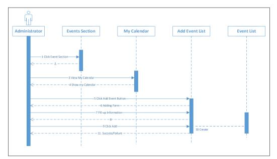
Figure 15. Sequence Diagram for Administrator's Account Setting Section
