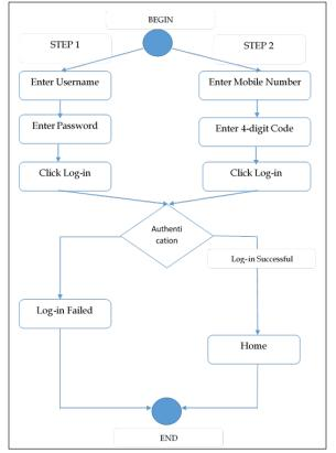
Figure 17. Activity Diagram for User Login Using 2-Step Verification Process
